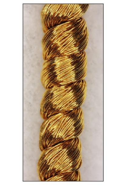
Electrode made of 100 strands of metal wire, twisted and then wrapped around an inner core.
