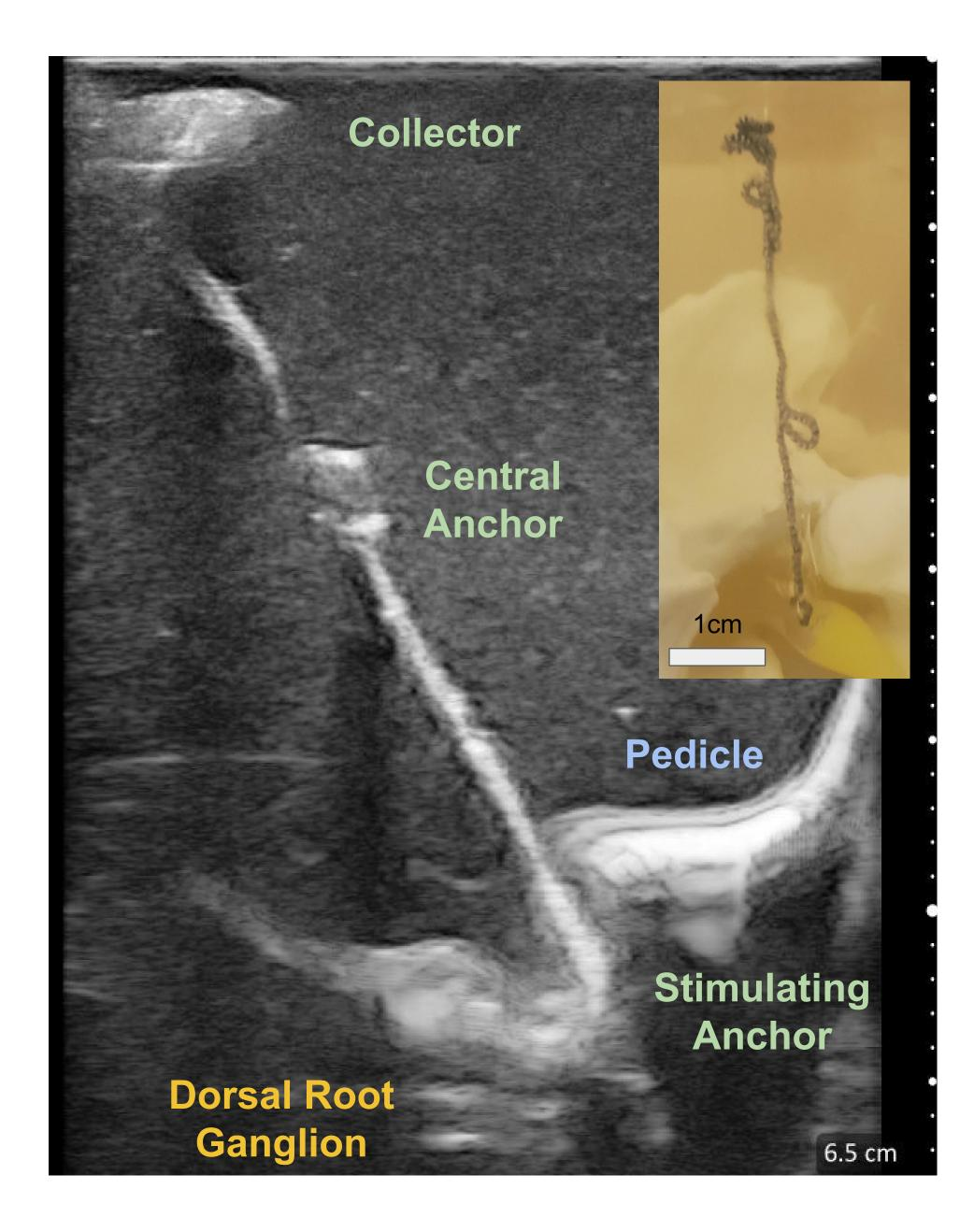
Figure 3: Visualization (Clarius L15HD3) of an injectable electrode placed in a gelatin model, where the hyperechoic backscattering agent (silica powder) highlights the characteristic acoustic shadow cast by the device. Modeled bone and nerve anatomy is also seen. An image of an injected electrode placed in such a semi-clear gel is provided in the insert.
