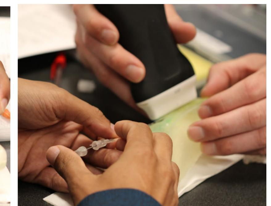
Figure 2: A gelatin model of the wrist with embedded anatomical components used to training both visualization of the needle and placement of the injectable electrode. Shown here is the Clarius L15HD3 using an in-plane approach.
