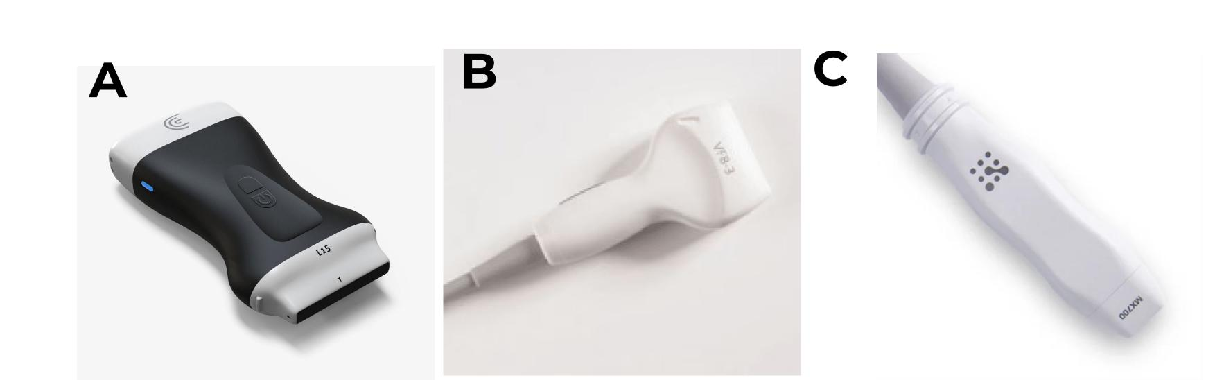
Figure 1: Ultrasound probes used in this study. A: Clarius L15HD3; B: Acuson VF8-3; C: Vevo 3100 MX700. A and B are clinical units, whereas C is a research use only ultra-high frequency system capable of visualizing nerve fascicles.
